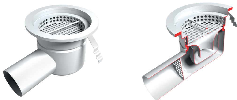
MSG110-BR Spot Gully Type 'B' c/w 110mm Side Outlet Round Flange incl Foul Air Trap (FAT) & Trash Basket
