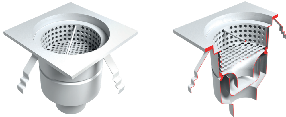
MSG110-BR Spot Gully Type 'B' c/w 110mm Side Outlet Round Flange incl Foul Air Trap (FAT) & Trash Basket
